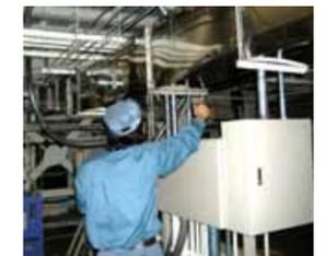
Duct leakage measurement
