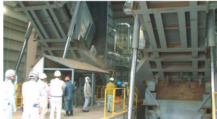
We enclosed the entire device in the building, and collected dust. As a result, the dispersion of dust in the building disappeared almost.
